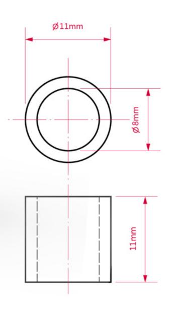
This dimension of racing ring is fit for GPS tracker ring.
